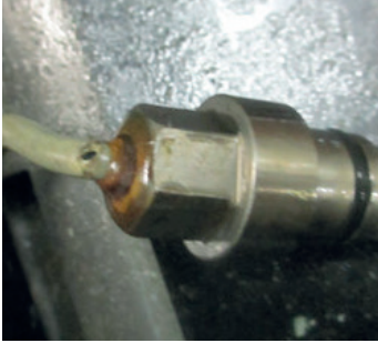
Fig. 2a: Defective feedback sensor
