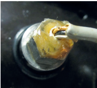
Fig. 2b: Defective feedback sensor
